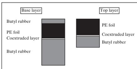
Fig. 4: Set-up of the corrosion protection tapes
