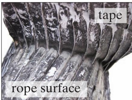
Fig. 5: Adhesion and gearing of the base layer to the rope surface
