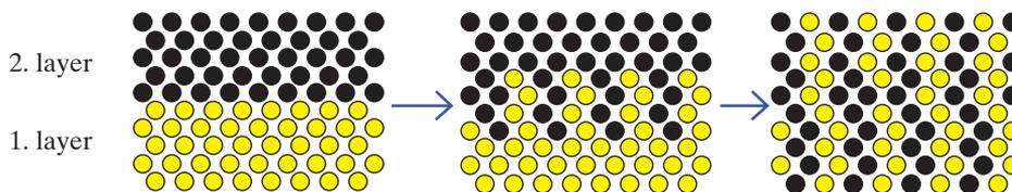
Fig. 3: Cold welding of the butyl rubber tapes
