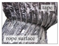
*Fig. 5: Adhesion and gearing of the base layer to the rope surface*
